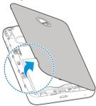
Find the notch on the lower left side of the back cover. Use your fingernail to open the back cover and lift it up gently.
