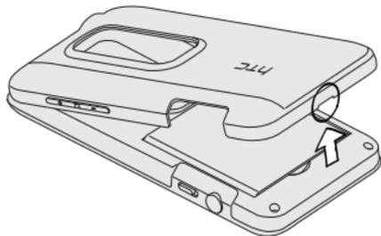
2. Lift the battery out at the notch at the bottom of the battery compartment.
