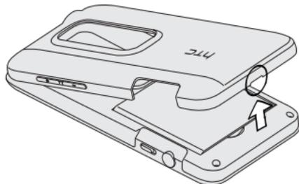
2. Insert the contact end of the battery first, and then gently push the battery into place.
