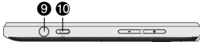
9. **Camera button** Launches the camera and functions as a convenient shutter release and record button.
